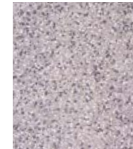
Exposed Aggregate Concrete
